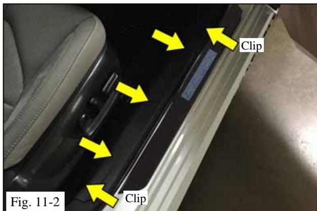
(c) Make sure the clips on either end of the sill trim engage properly (Fig. 11-3).
